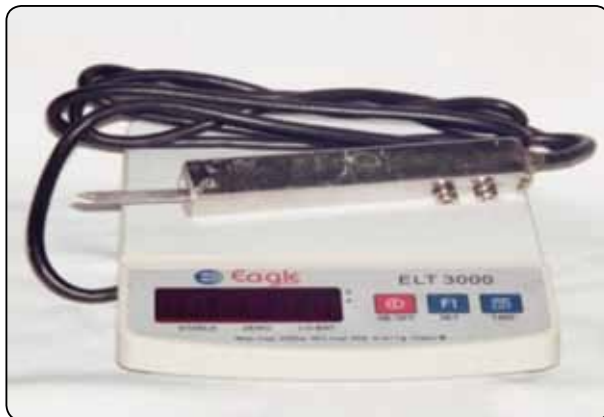
Fig. (6): The retention testing device
